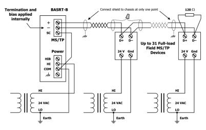
Figure 9 — 2-wire MS/TP Bus with Separate Power Sources
