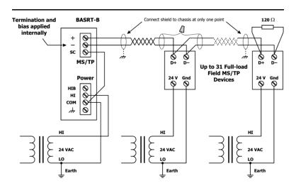
Figure 10 — 3-wire MS/TP Bus with Separate Power Sources
