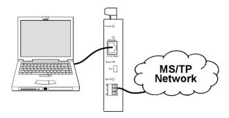
Figure 12 — Setup for Initial IP Address Configuration
