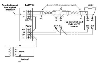
Figure 7 — 2-wire MS/TP Bus with Shared Power Source
