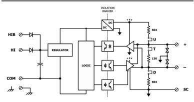
Figure 11 — Isolated EIA-485 Transceiver Circuitry
